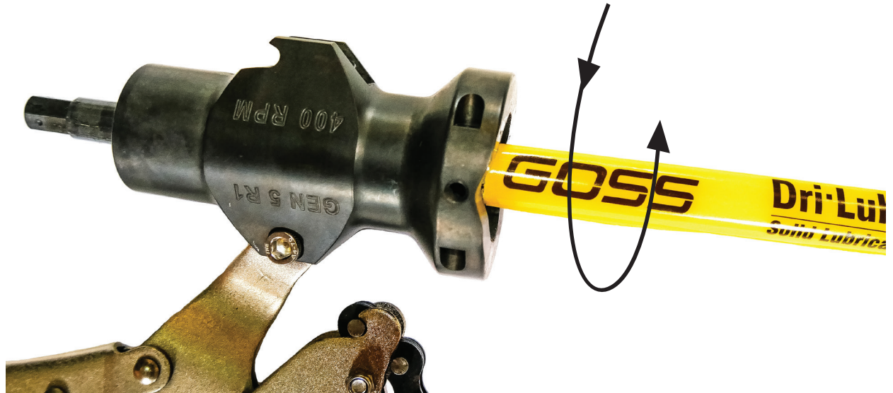
Fig. 5.1 IMPORTANT! Lubricate the cutters before drilling each hole. A light twist action will supply a sufficient amount.
