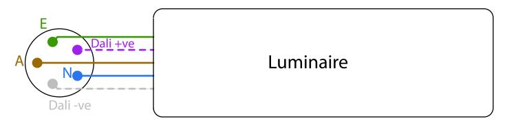
Note for non-dimming versions of the Product: the Dali +ve, and -ve cables are redundant and do not need to be connected.
