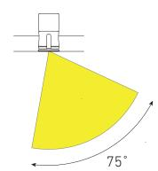
Elliptical asymmetric distribution displayed here with a vertical mount.
