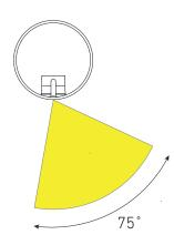
Elliptical asymmetric distribution displayed here with a vertical mount.
