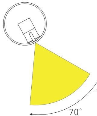
Elliptical symmetric distribution for typical mounting at 30° from vertical.
