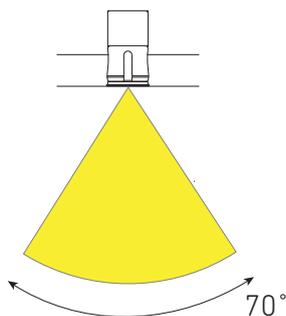
*Elliptical symmetric distribution displayed here with a vertical mount.*
