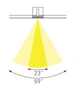
Circular distribution measured at vertical down (0°) mounting.
