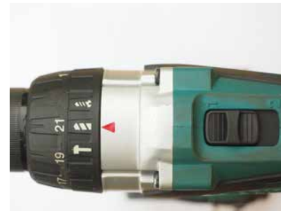
Above: Our example drill is set to: "Drill"; high torque; and LOW speed (1)
