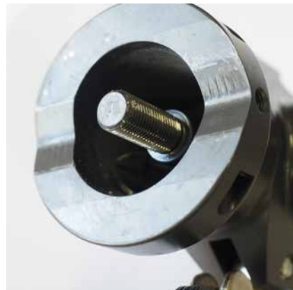
Fig. 2.2 Cutter end of the cutter assembly pictured above. The cutters are not yet installed. Proceed to cutter installation (step 3).
