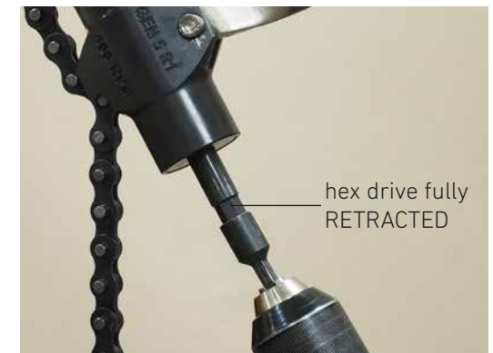
Fig. 8.3 Set drill to reverse and back out the cutters / hex drive until it is fully retracted.
