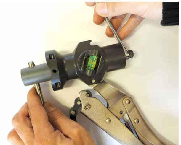
Fig. 3.4 Use the cutter removal tool and spanner provided to remove or secure the cutters. Note the cutter removal tool's 15mm side (shallow) and 16mm side (deep).
