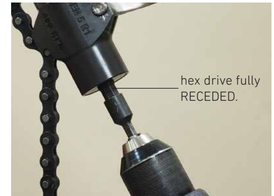
Fig. 8.2 STOP drilling once the hex drive has fully receded inside the Drill Jig.
